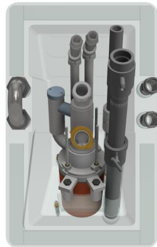
BURNER INSTALLATION IN JETBOX
