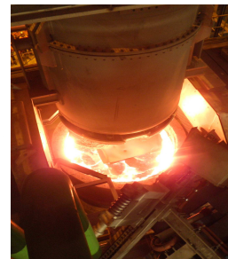
200t RH - plant with mechanical pumps Saarstahl, Germany
