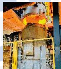
8t DETEM VD-VOD plant with mechanical pumps NPO, Russia
