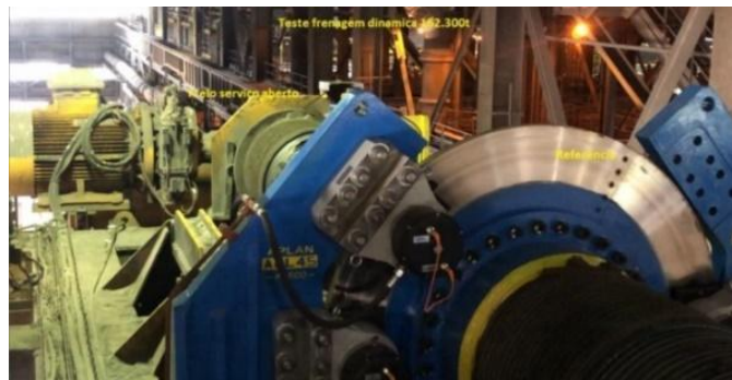
Figure 20. Dynamic braking 162.3t - service brake off.
